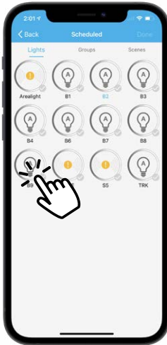
Using the "Scheduled" button, Select the light/group/scene that needs to be scheduled and press the "Done". Use the "Auto/On" or "Off" buttons to define the logic of the schedule.
