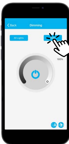
Access the Dimming page for lights/groups within the zone. Click on the wattage button to edit the power rating
