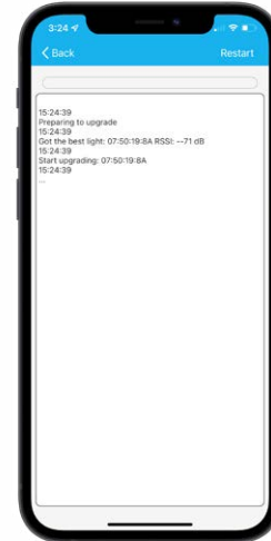
The progress of the mesh upgrade is shown on a separate page. Check if all lights have been upgraded successfully. The restart button can be used in case of any update failures.
