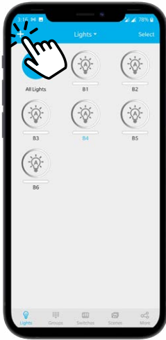
Press the “+” icon to add lights. The lights that can be added to the current zone will show up on the screen
