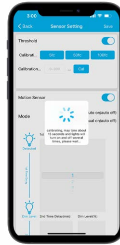
Fixture will blink a few times as part of the calibration process. Calibration is done when fixture stops blinking.
