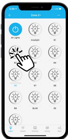
To rename a light, long press the light icon and the Light Dimming page should appear
