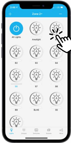
Long press the light icon to open up the individual light dimming settings.
