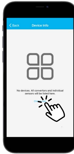
Use the "Click to Add" button to search for the Energy monitoring device
