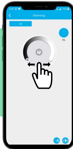
Adjust the dial to control the brightness. Tap the gear icon at the bottom right to access Sensor settings
