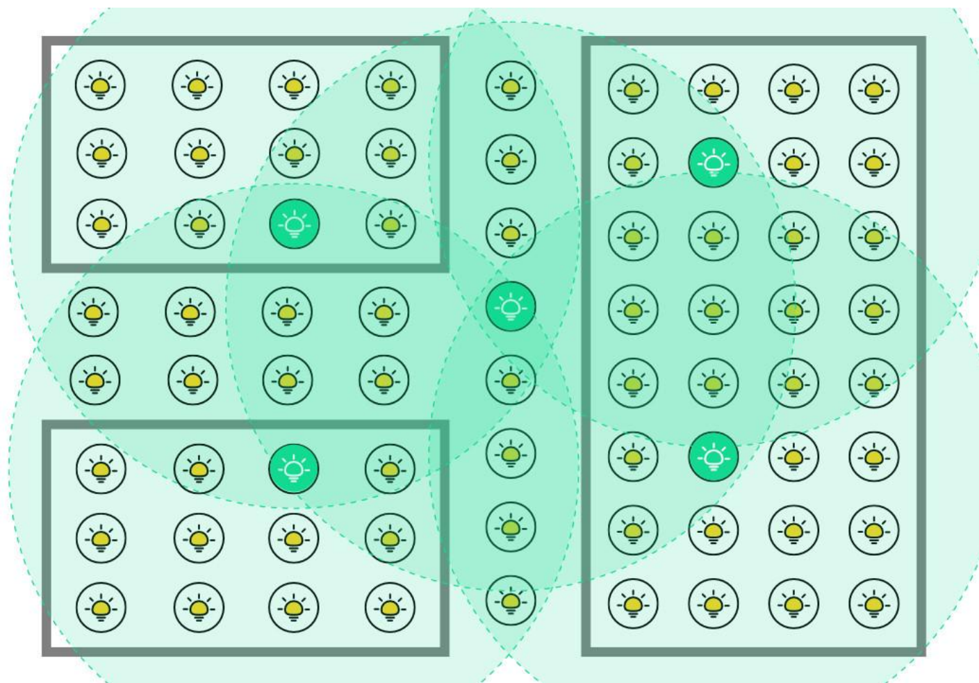
Fig. 1. Example of relay placement in a dense, grid network layout
