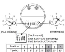
The potentiometer T sets the period of delay time that sensor will turn off the connected lights after the area is vacated.
