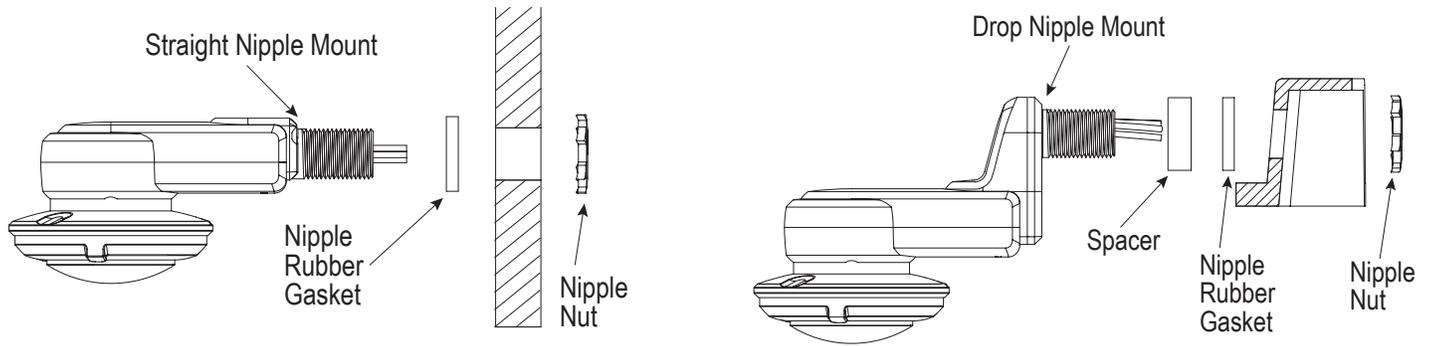
**NOTE:** The Outside Fixture Wall thickness should be no greater than 0.125" (3.18mm) for optimal sensor mounting and security.
