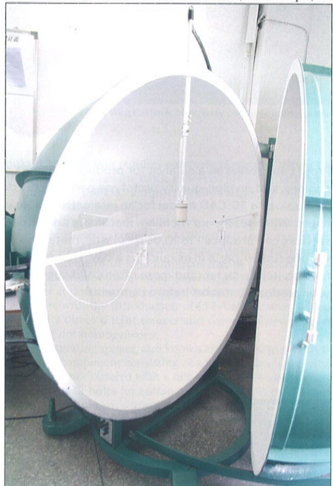
Example of a large integrating sphere used to measure transmittance and reflectance. ("Luminance Chamber" by Swoolverton)
