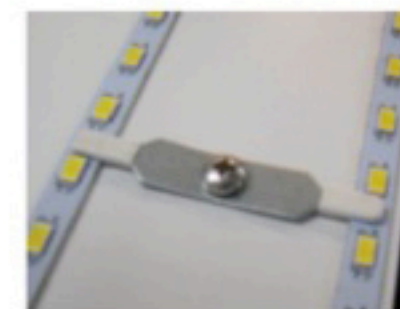
Multiple hold down clips ensure thermal contact and easy upgrade
