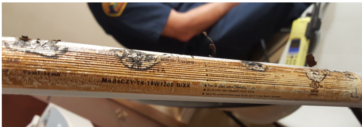
James Industry Dual-Mode T-8 Replacement Tube Model No. ZY-T8-18W1200 BIXX in which the HOA fire began (cause under investigation).
