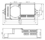
Mechanical structure (mm)
